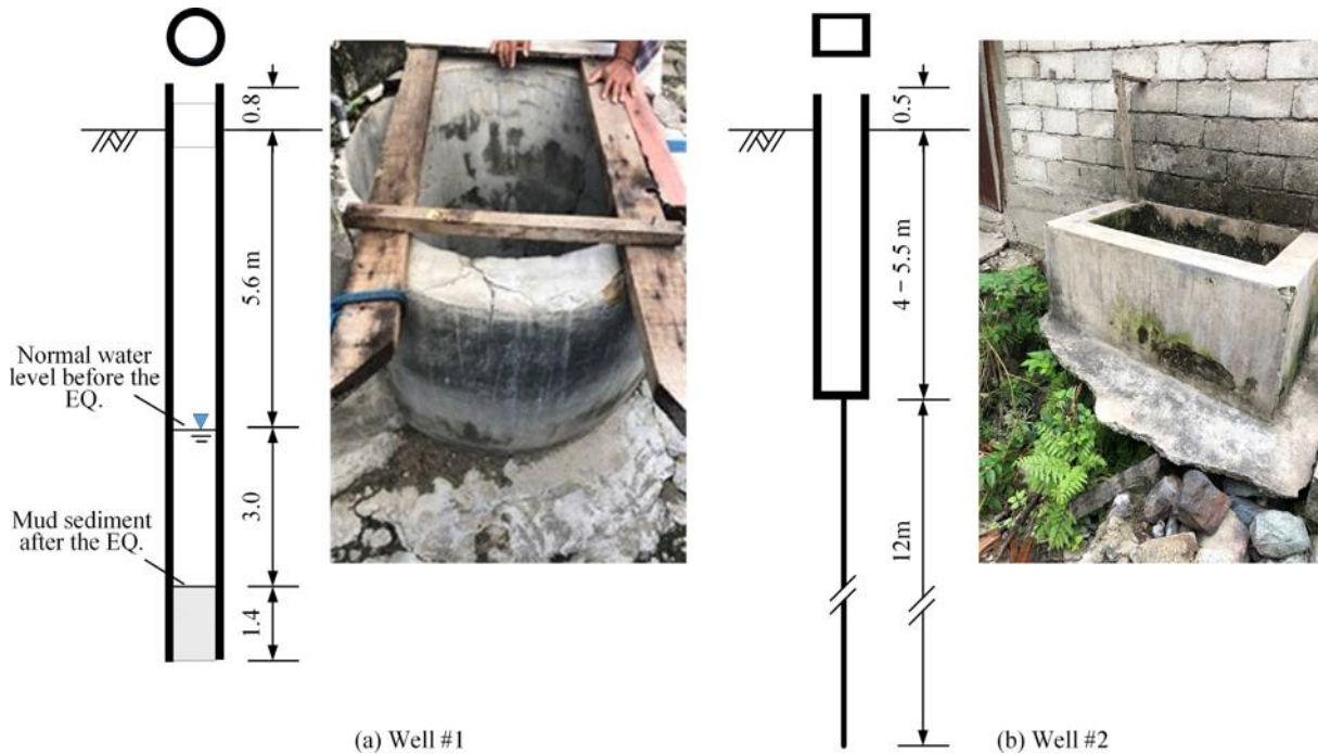
Fig. 2. Photos and cross sections of wells near flowslide area.
